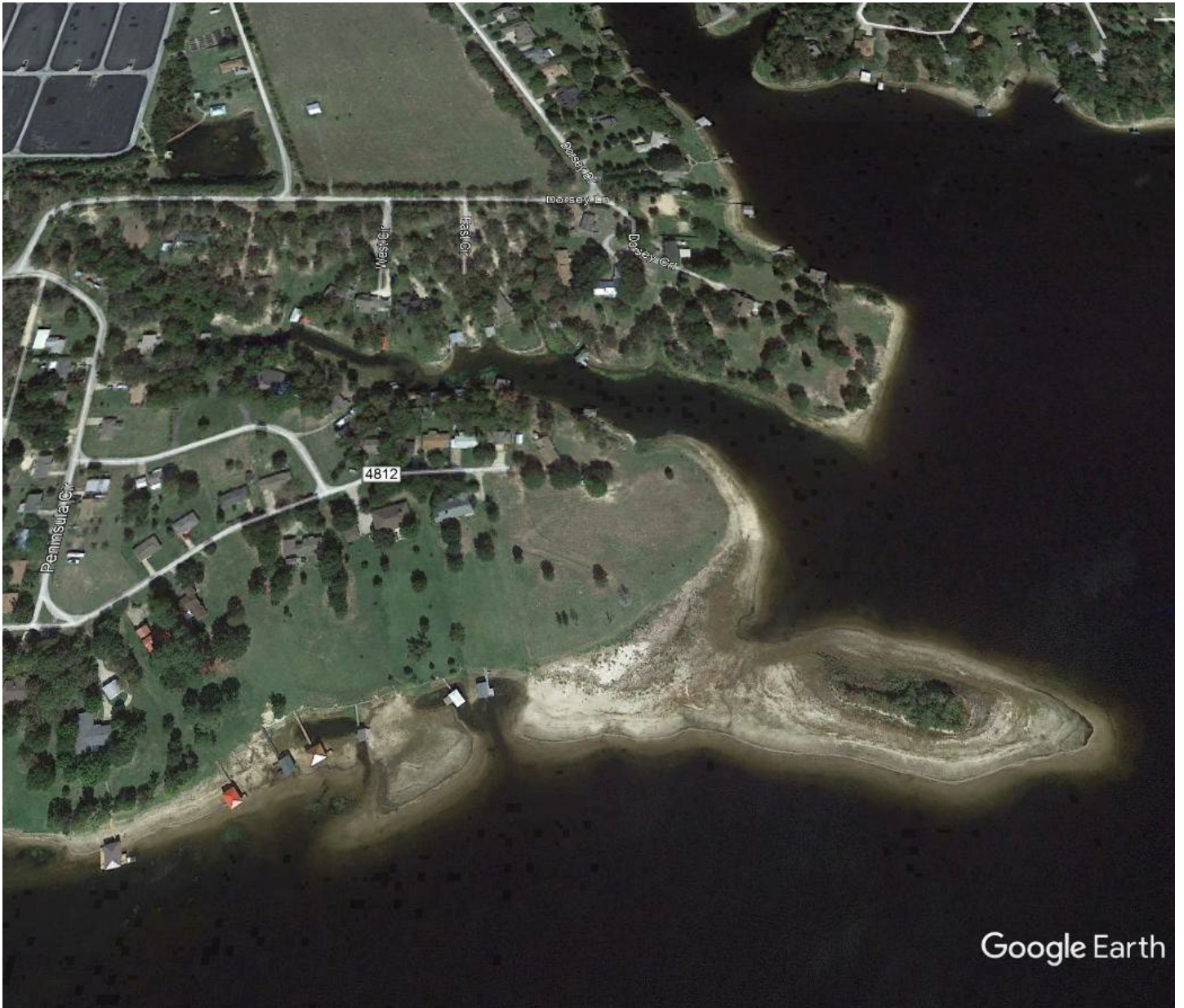
Figure 4. Google Earth image from October 17, 2012 showing extensive reservoir bottom exposure due to low water from the extended drought.
