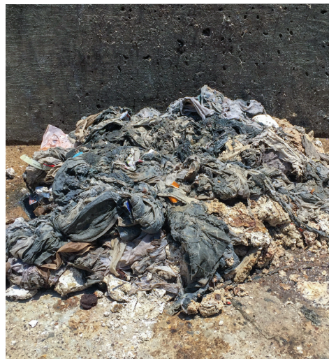
Rags and grease pulled from the system
